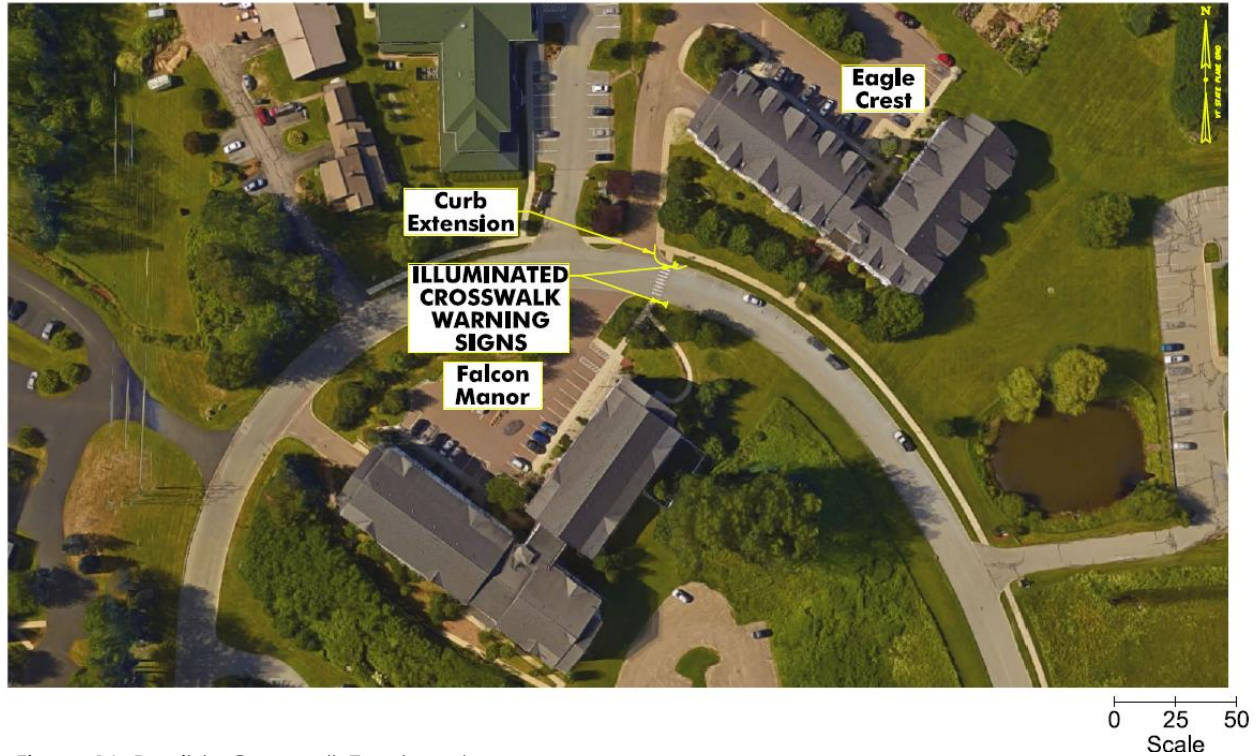
Figure 16 Possible Crosswalk Treatment
