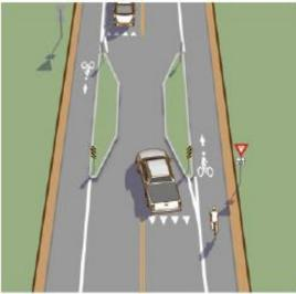
• Lateral shifts – This realigns an otherwise straight travel path and creates chicanes in effect. By forcing drivers to turn, this measure lowers vehicle speeds:
