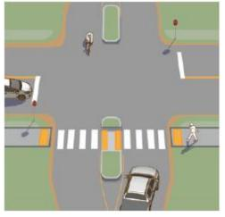
Striping, bollards and planters can be used to temporarily or seasonally implement high-impact traffic calming measures:
