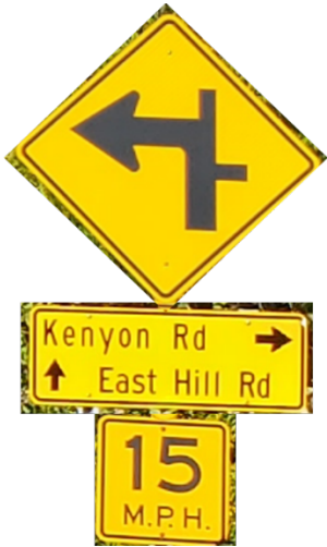
Figure 6: Revised turn signage assembly example
