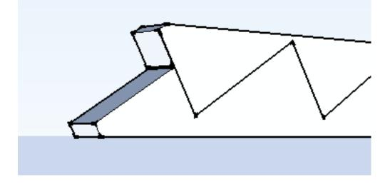
7.. **Cut the treads to length.** These cuts are important. Each tread must be the same length and cut square. Typically we make the treads 3' wide. The top tread needs to be at least 4" wider as it spans both stringers.
