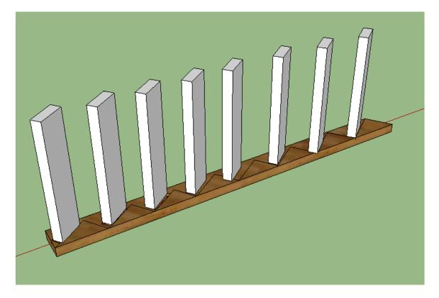
10. Place the second stringer on top. Working your way from one side to the next, ensure the treads are set in the notches. Affix the lag bolts and washers using an impact drill driver and a mallet. Flip the ladder over and repeat for the other side. The ladder is ready to install!
