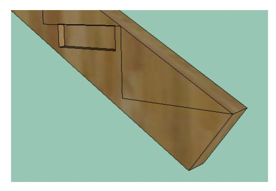
6. **Use a router to cut notches in the stringers.** For a 3x8 stringer, notches should be 1" deep. Test the fit with a block of wood. Use a chisel or multi-tool to clean up notches as necessary.
