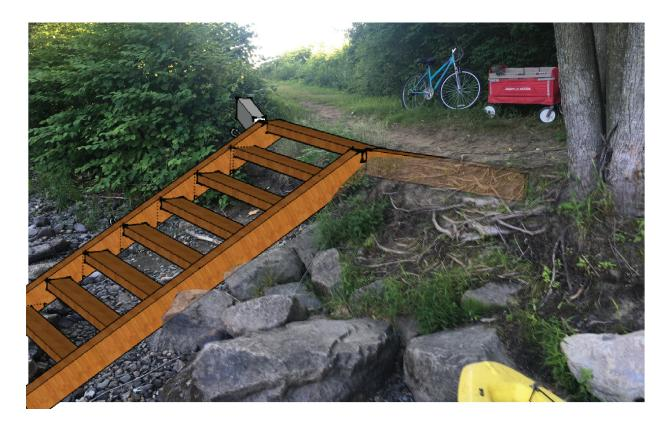
Typically the steps are built out of 3"x8" rough cut cedar, often sourced from Goodridge Lumber in Albany, VT. Treads are a minimum of 3' wide. A 5' wide step is preferred for launching boats, although larger staircases can be more unwieldy to install and remove.
