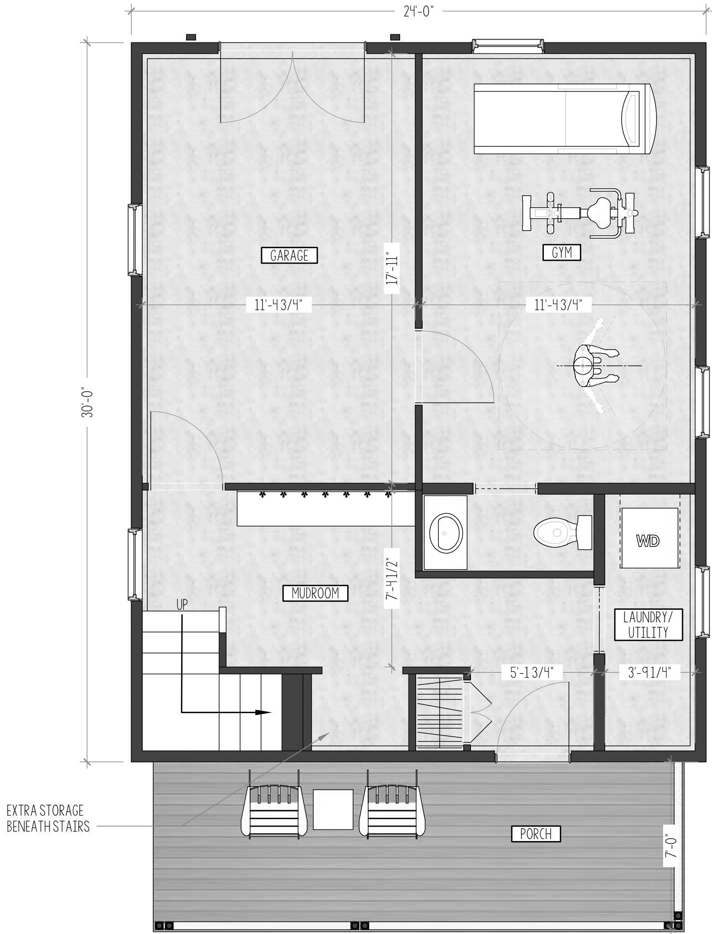
1 FIRST FLOOR PLAN SCALE: 1/4" = 1'-0"
