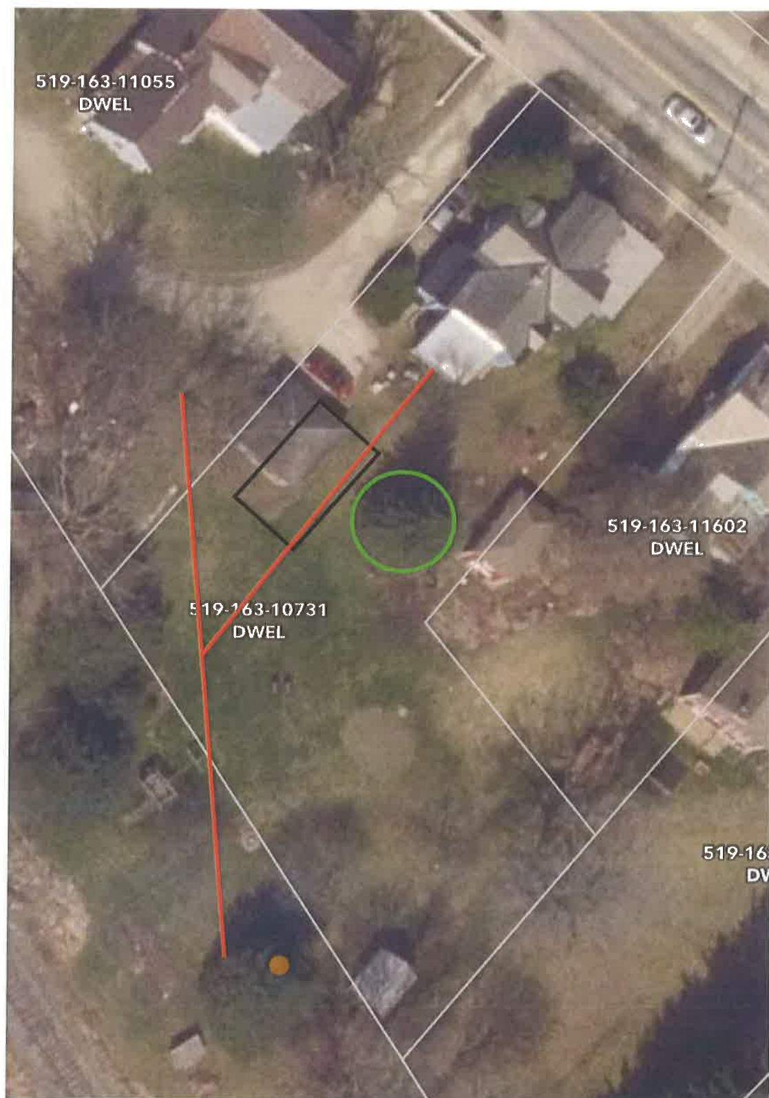
Figure 2: Black rectangle represents approximate footprint of proposed structure if sited 10 feet from property line. Red lines represent approximate location of sewer lines. Green circle represents approximate footprint of evergreen tree.
