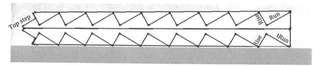
5. Make a block out of wood of the same cut as the treads. Use this to trace the locatons of the notches for everything but the top step. Be consistent with the locations of the notches (i.e. on the line, but one inch in from the edge). Note: rough cut lumber varies – measure each piece of lumber before deciding what block – or blocks – to use for tracing.
