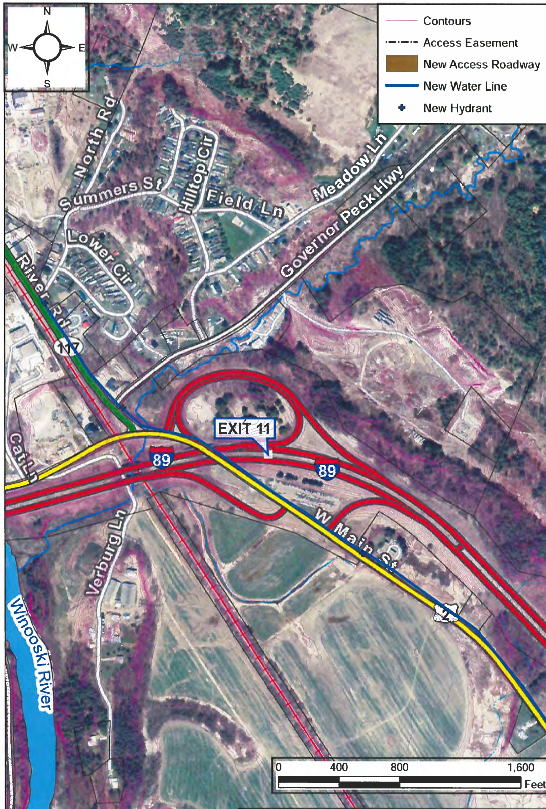
Figure 4A Proposed Waterline Extension - Phase III Town of Richmond Access Road With Water and Sewer Extensions for West Main Street
