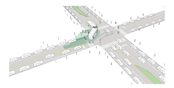
Articulated buses, or extended coaches pivoting around a center bridge plate, are most commonly 60 feet long. They are generally the assumed operating vehicle in BRT or "open BRT" systems.
