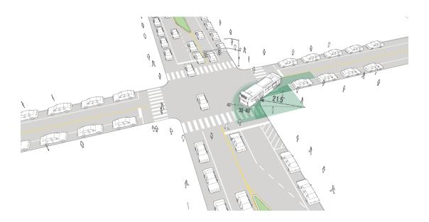
A typical inner turning radius of a standard 40-foot bus is 21.5 feet, which is required to clear the curb. At its tightest turning angle, the rear overhang of the back bumper extends out to 43.3 feet.
