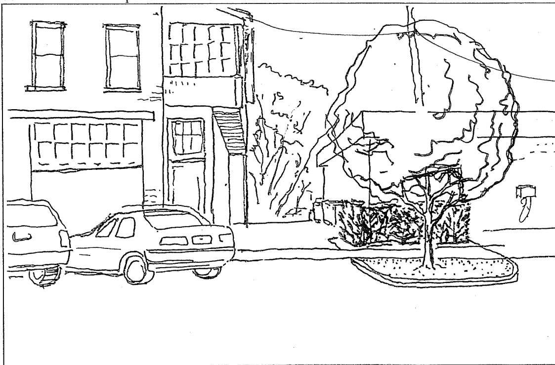
Proposed Green space and sidewalk added to Bridge Street right-of-way- Tree provides shade and screens pole. Hedge (or fence) screens dumpsters. Sidewalk indicates pedestrian route.
